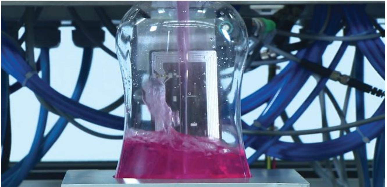
At the German Research Center for Artificial Intelligence, the RFID chip (seen close up on the back of the bottle being filled) and Siemens hardware are used to communicate instructions to the production equipment for proper processing and quality verification. Image courtesy of Siemens PLM Software.
