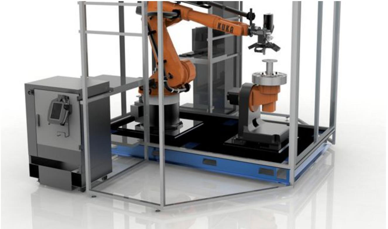
**The Robotic Composite 3D Demonstrator from Stratasys uses a robotic arm with an extruder for greater motion control. Image courtesy of Stratasys.**
